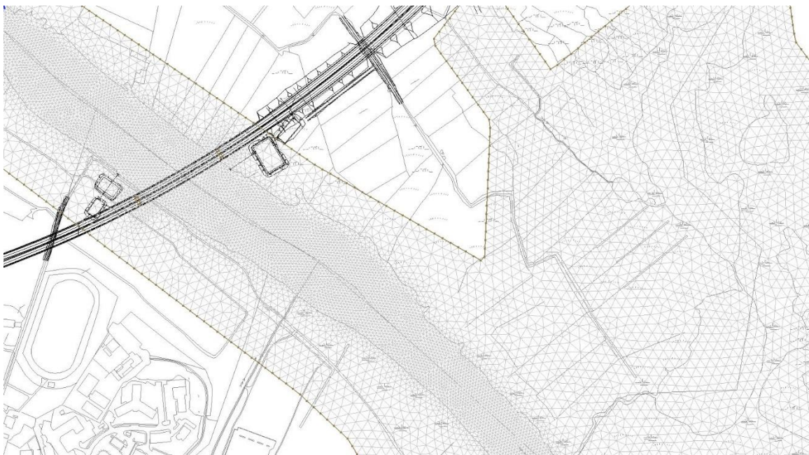
Figure 9 Model Grid Density in the vicinity of the River Corrib Bridge crossing
